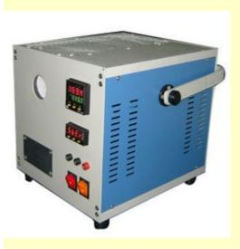
We offer best quality High Temperature Dry Calibrator that are made using nest grade raw material. Also known as DPI-1200, these are furthermore highly appreciated for portability and light weight. The rugged features of these products makes them highly sought after in the petrochemical and pharmaceutical industries. Our calibrators are used for testing thermometers and sensors ranging from  $200.0 \sim 1200^{\circ}$ C.
